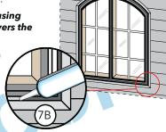
Note: This method creates a more flexible sealant line capable of expanding and contracting.
